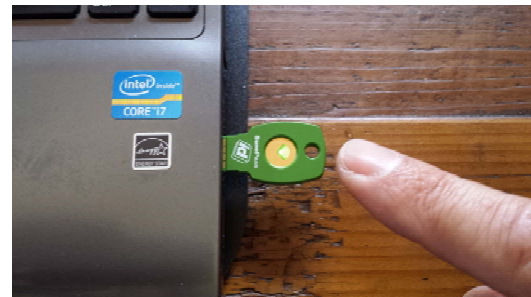
TapID Treo USB FIDO Key – touch to send FIDO code; touch to send OTP (it knows which to send)
